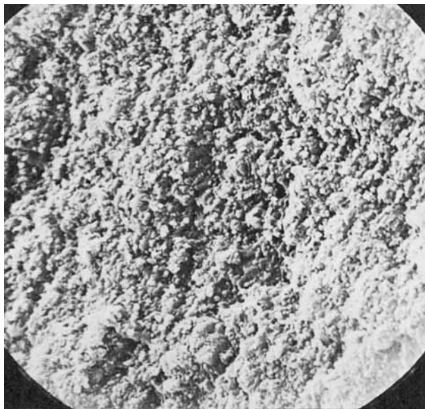
Fig. 6. SEM picture of the internal surface of fractured polymer 3 ( \times 3000 ).
